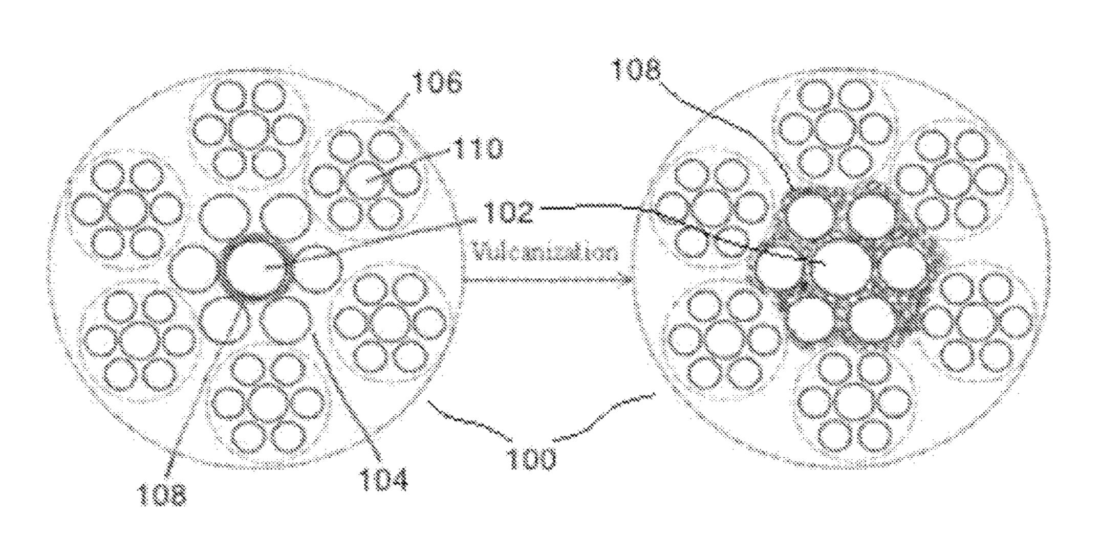
sheets are formed from a polymeric material with resilient properties. In some aspects, the volume of the coating after vulcanization is from 30 to 5000% higher than prior to vulcanization. The coating may contain at least one of a blowing agent and/or microbeads.
