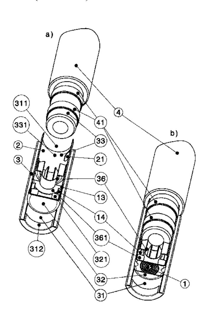
vaporizer membrane are arranged orthogonally or at an angle to the direction of the fluids passing through the mouthpiece.
