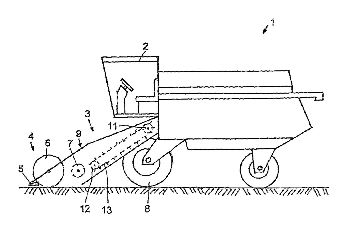
for the harvested crop. That is because the cross section of each of the carrier bars viewed in conveying direction, occupies at least 30% of the smallest internal cross section of undershot conveying duct.
