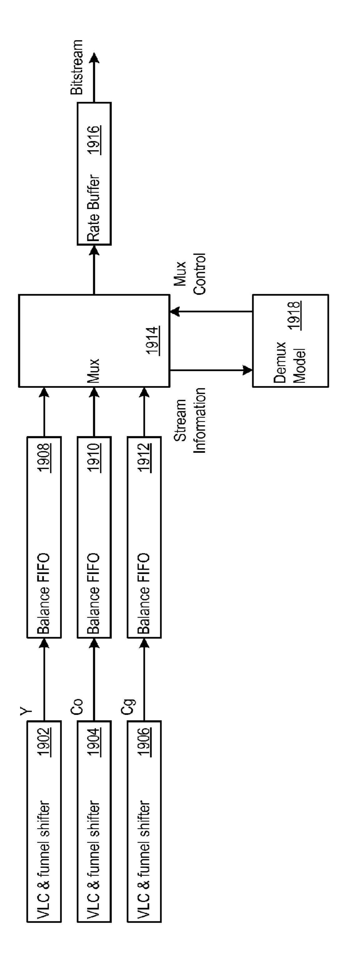
Mux puts mux word from each substream into bitstream when its model of decoder funnel shifter has space for a mux word. Can mux 0, 1, 2, or 3 mux words each clock cycle.
