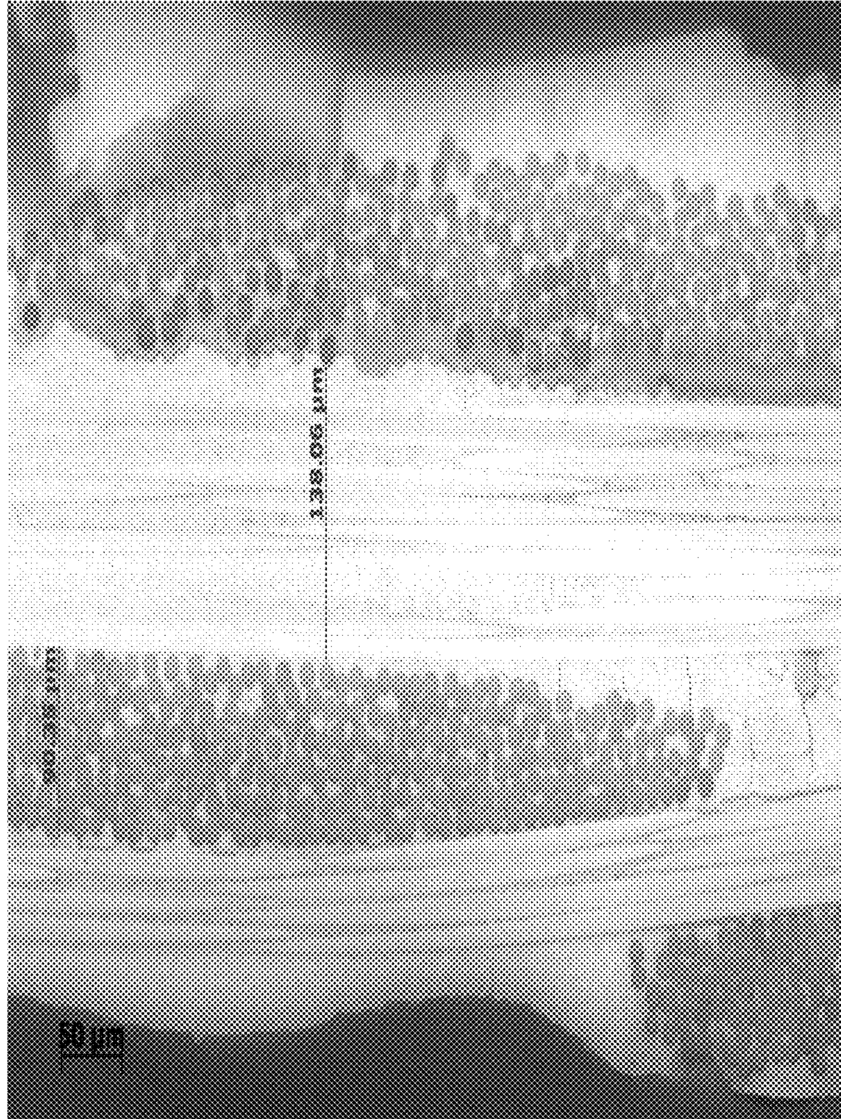
Fig 12. Oxide-oxide composite cross section 50micron
