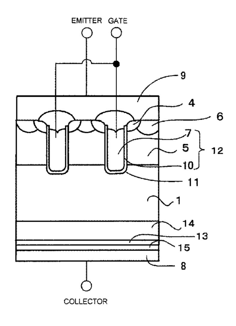
impurity concentration of the p<sup>+</sup> type collector layer, can be included between the n-type field-stop layer and p<sup>+</sup> type collector layer.
