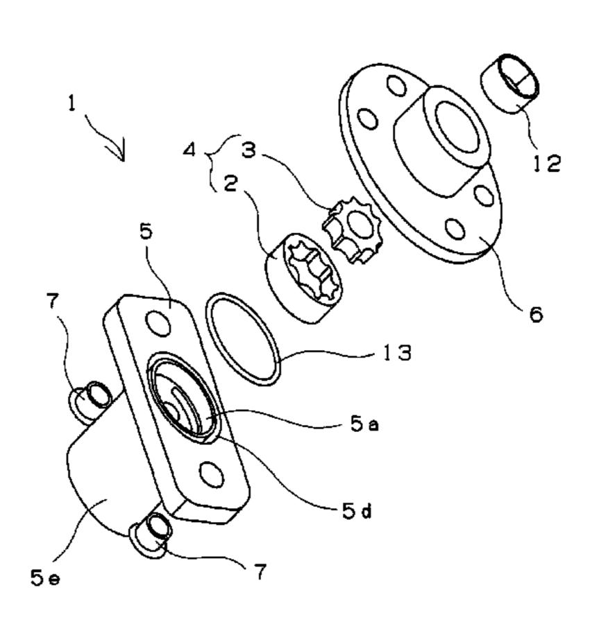
trochoid 4; and a cover 6 for closing off the recess 5a of the casing 5. At least some of the casing 5 is a body injection-molded from a resin composition. The invention also comprises a groove 5d in a portion of the recess 5a of the casing 5 in which the outer periphery is sealed, with a sealing ring 13 installed therein, and bushings 7 made from sintered metal that are provided integrally during injection molding in bolt fixing hole portions.
