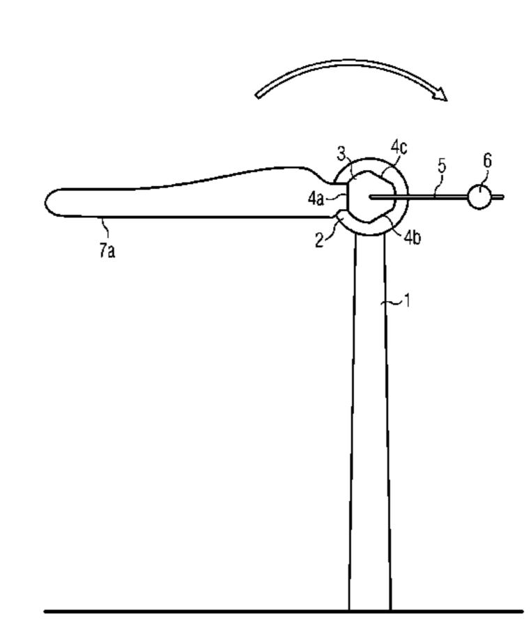
arrangement and the counter weight are rotatable in respect to the hub into a certain predetermined position.
