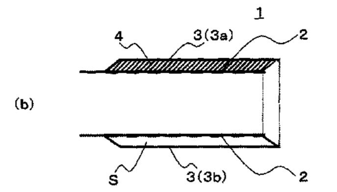
The distance between the exhaust pipe and the tubular heat shield plate in an area in which the closed space is formed is 1 to 50 mm.
