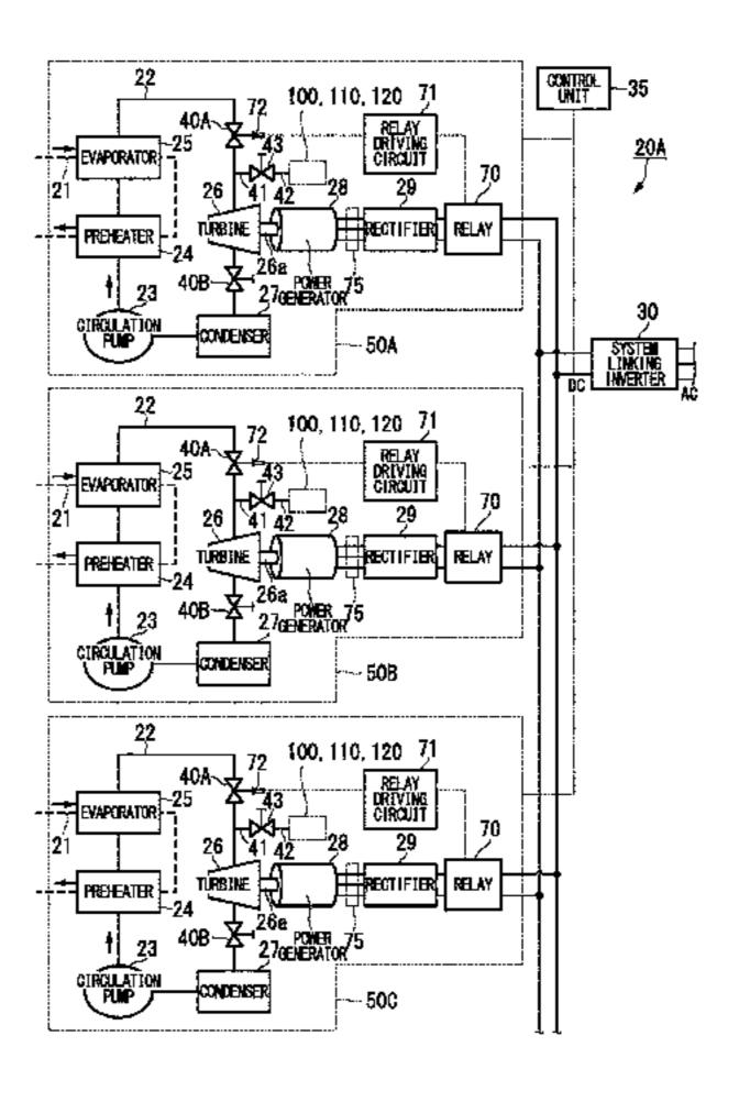
system (30), an operating unit (40A, 40B) configured to be operated when maintenance starts, and a relay driving unit (71) configured to interrupt power between the power generator (28) and the external power system (30) by the relay (70) when the operating unit (40A, 40B) has been operated.
