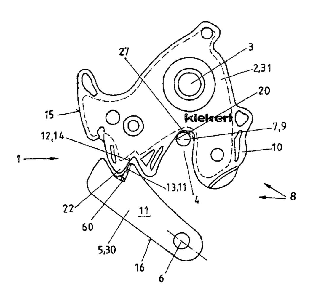
pawl, and subsequently are provided with a covering while maintaining the catch surfaces. After stamping, the locking parts are bent in the region of the main latch and/or another latch resulting in the formation a contour which is void of stamped channels, and are then inserted into the lock housing box.
