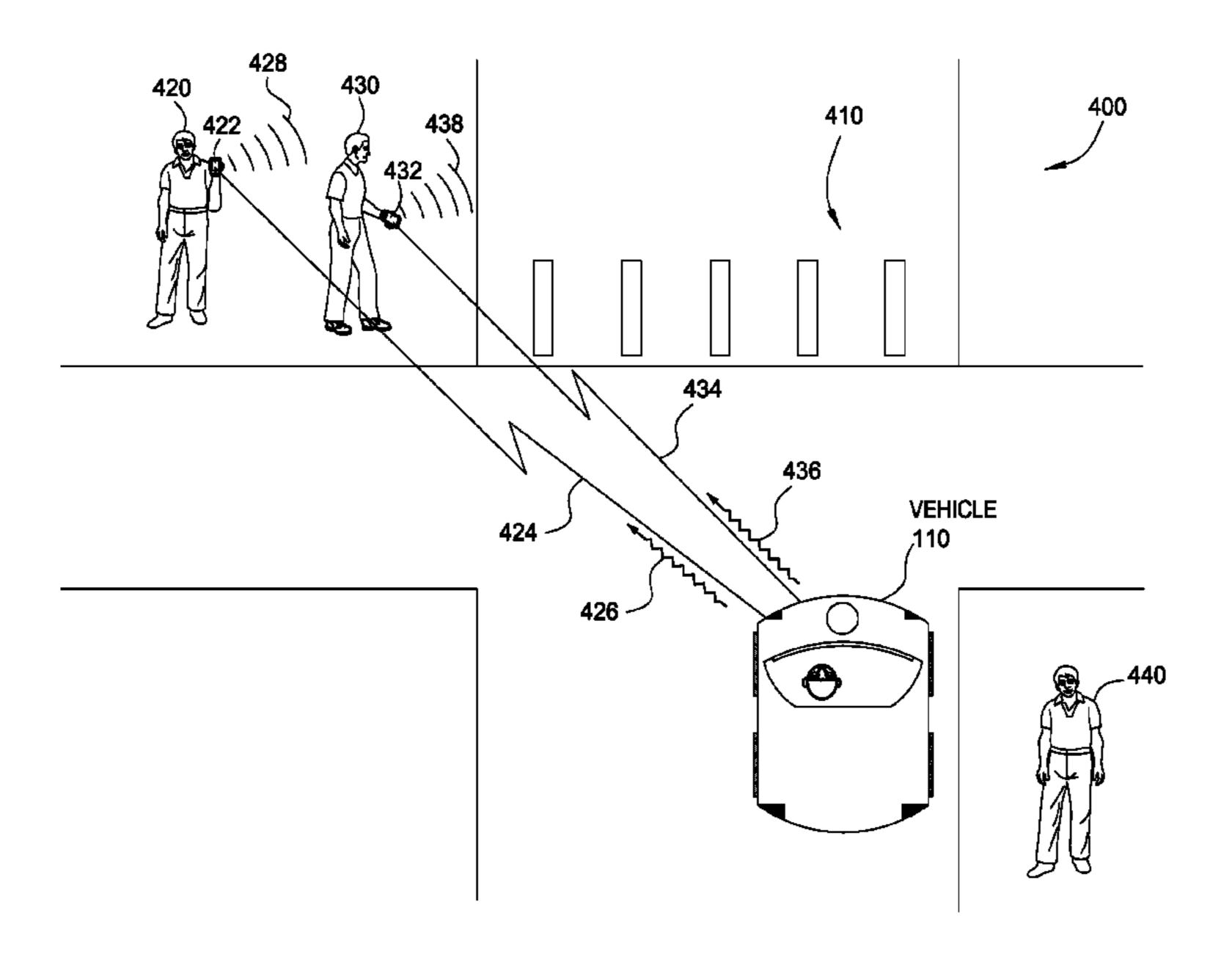
interest. The directional alert system may also wirelessly pair with computing devices residing in a target region associated with the direction of interest, and transmit wireless notifications to those computing devices to alert the users of those devices.
