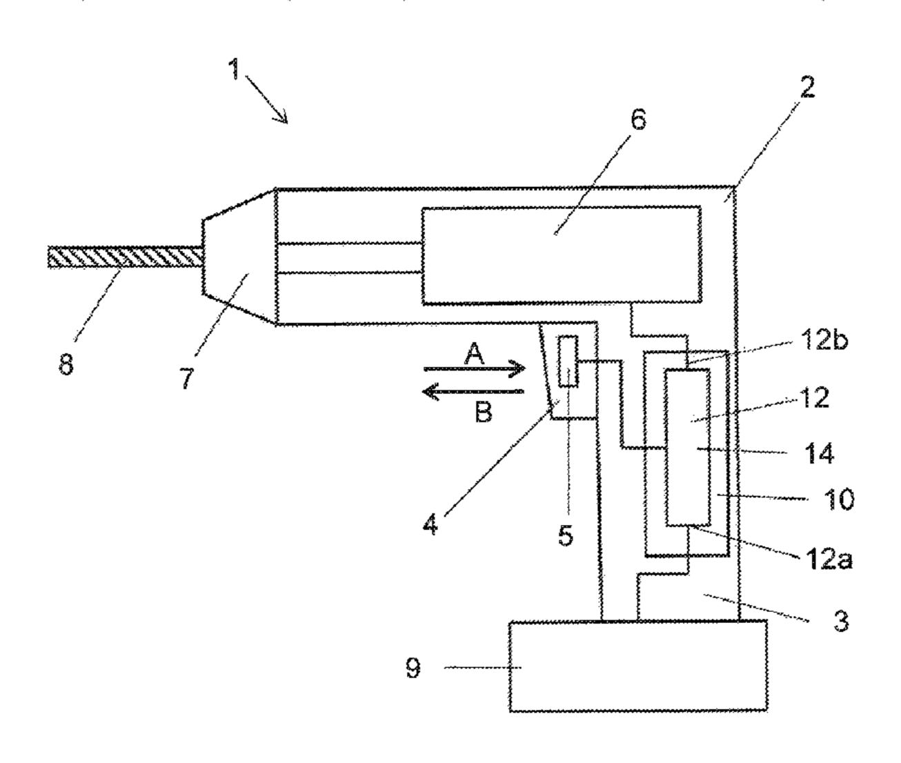
second value is selected for the PWM duty cycle, if an operation-value of the battery lies above the monitoring operation-value limit.
