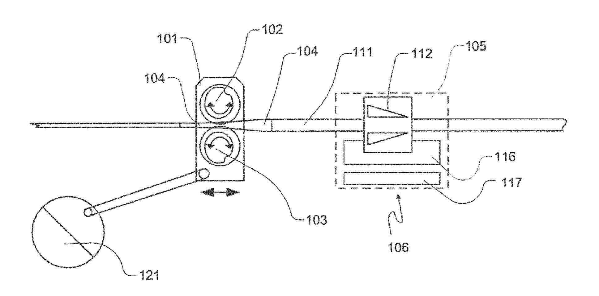
outer tube wall by applying liquid or solid CO<sub>2</sub> onto the outer tube wall in order to remove a contaminant from the outer tube wall.
