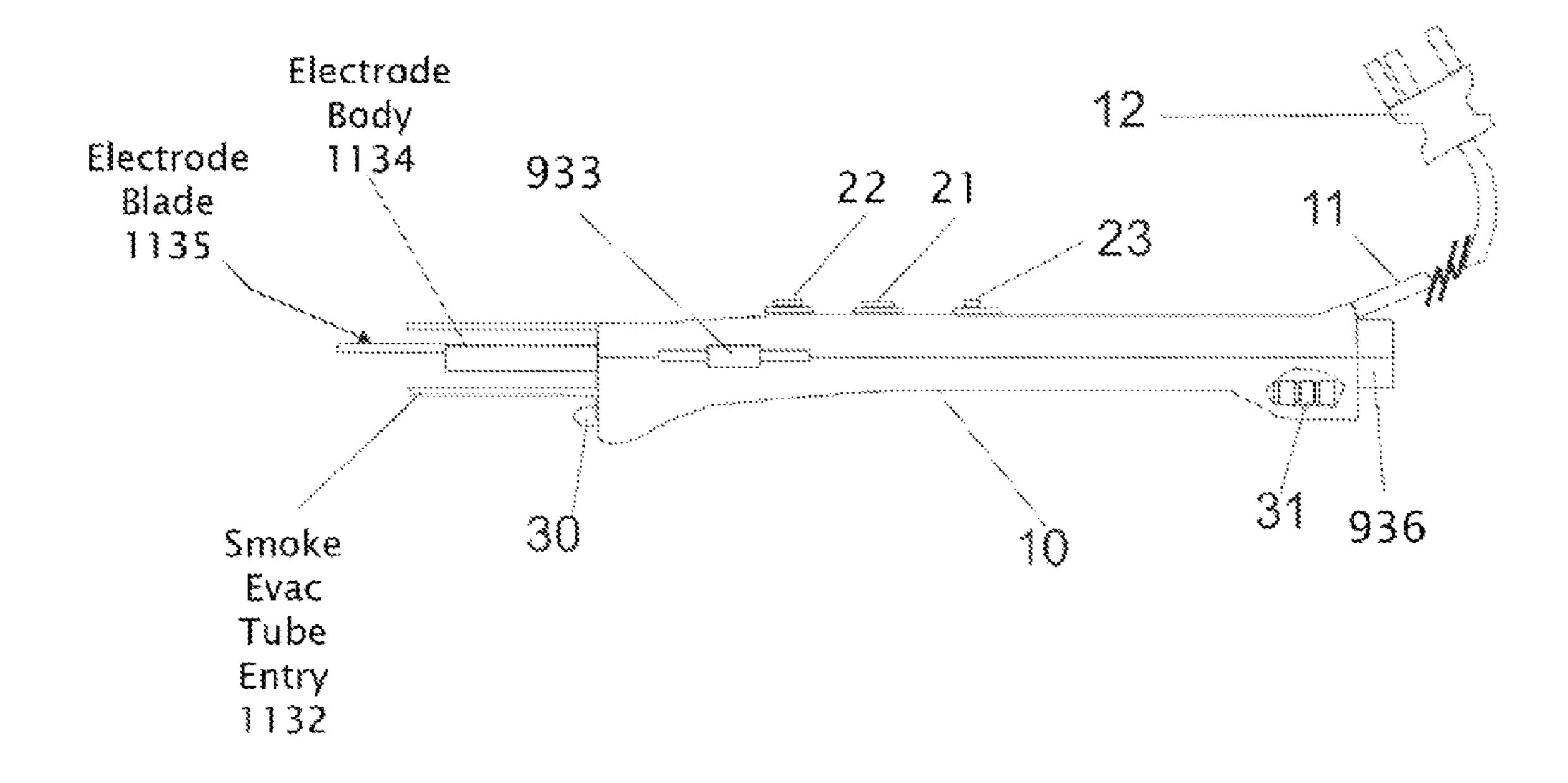
Exterior side view of an example of a fume evacuating electrosurgical scalpel with a fixed blade 1100
