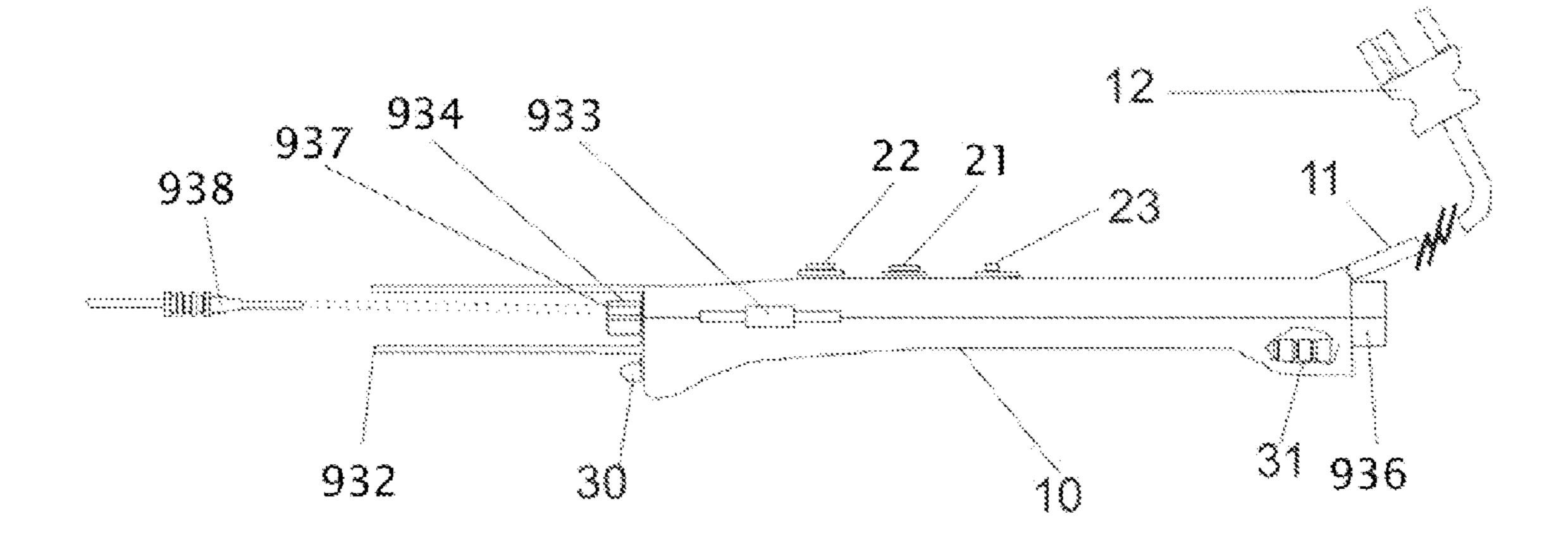
External view of fume evacuating electrosurgical scalpel with a removable blade
