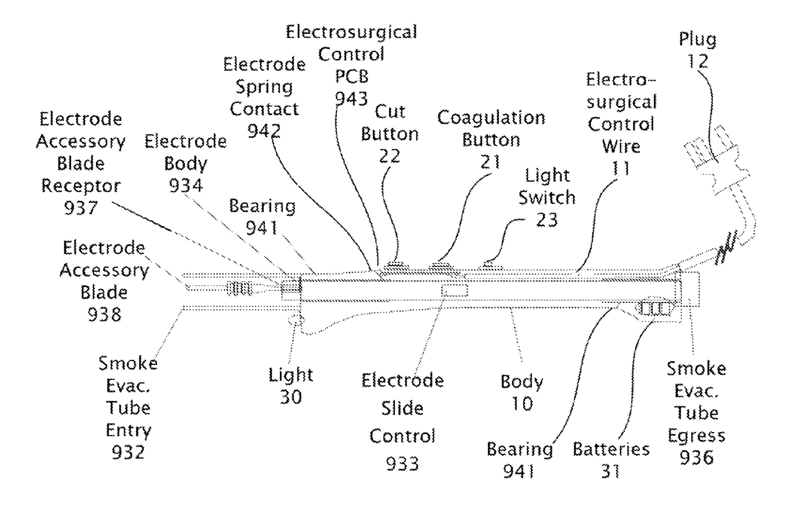
Internal view of fume evacuating electrosurgical scalpel with a removable blade
