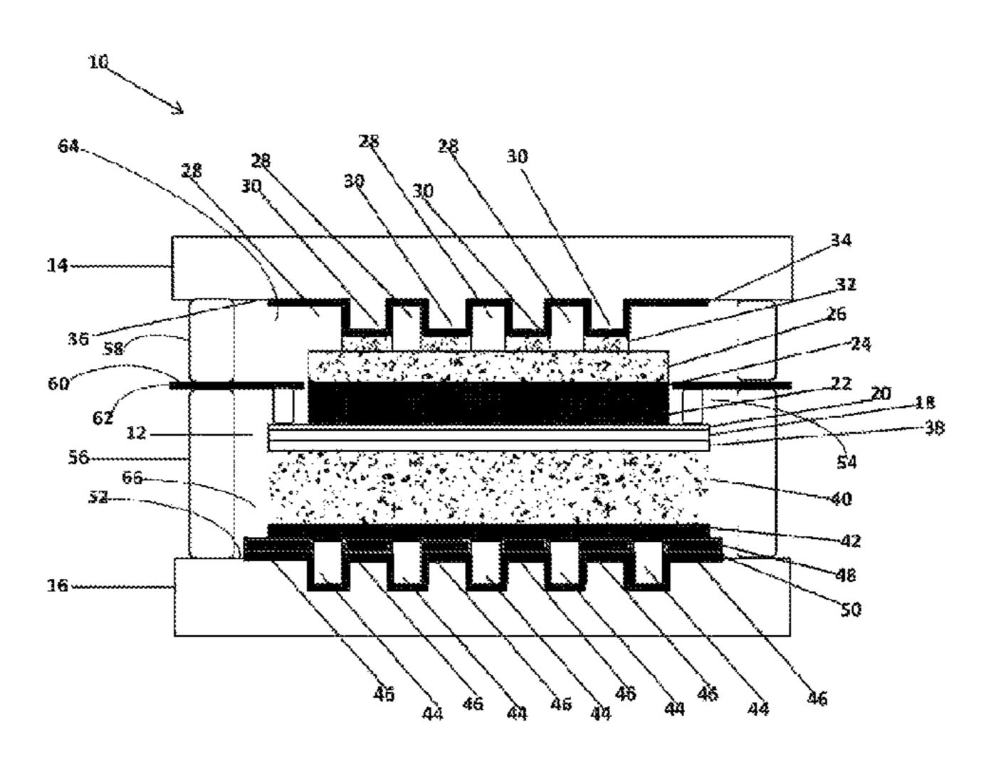
a gas chamber **64** between the cell and the gas separator. The invention also extends to the treated cell **12**.
