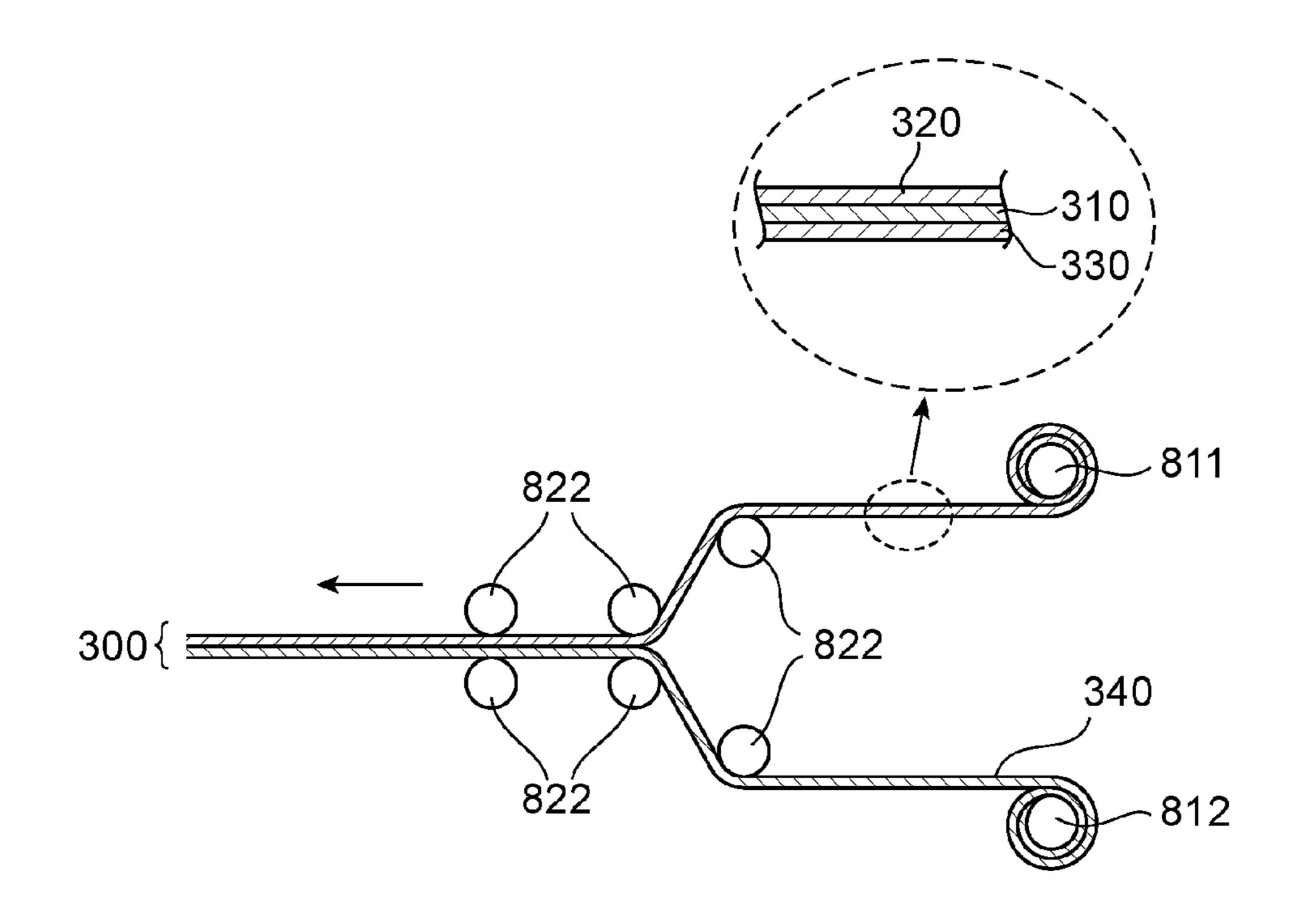
METHODS FOR PRODUCING PHASE-DIFFERENCE FILM AND CIRCULARLY POLARIZING PLATE INVOLVING SIMULTANEOUS REDUCTION OF CLIP PITCH ON ONE SIDE AND INCREASE OF CLIP PITCH ON ANOTHER SIDE
