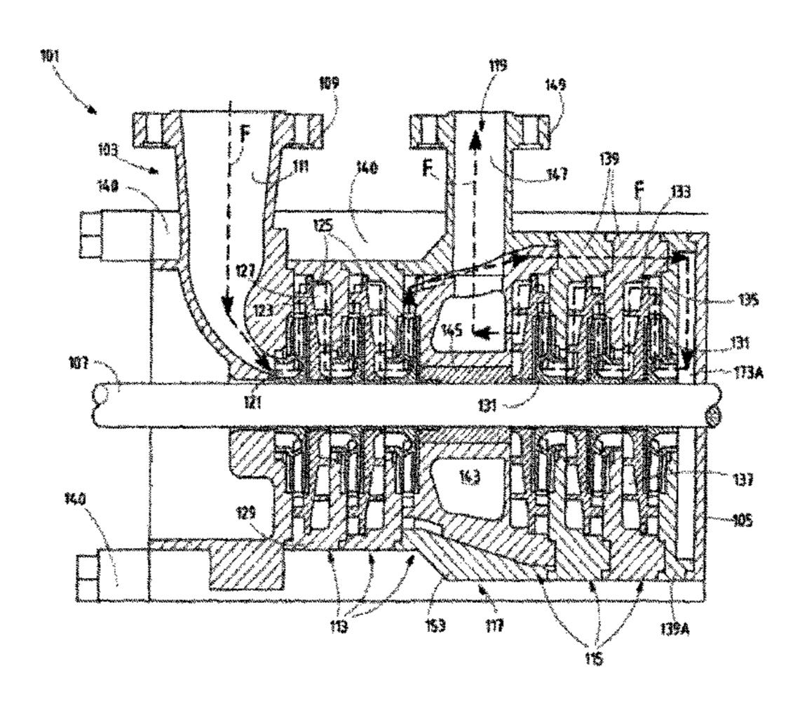
connection between the set of second stages and the pump outlet. The second diaphragms comprise each at least one peripherally arranged through aperture. The through apertures are aligned to form at least one passageway, which fluidly connects the axial transfer channel with a most upstream one of the impellers of the second set of stages.
