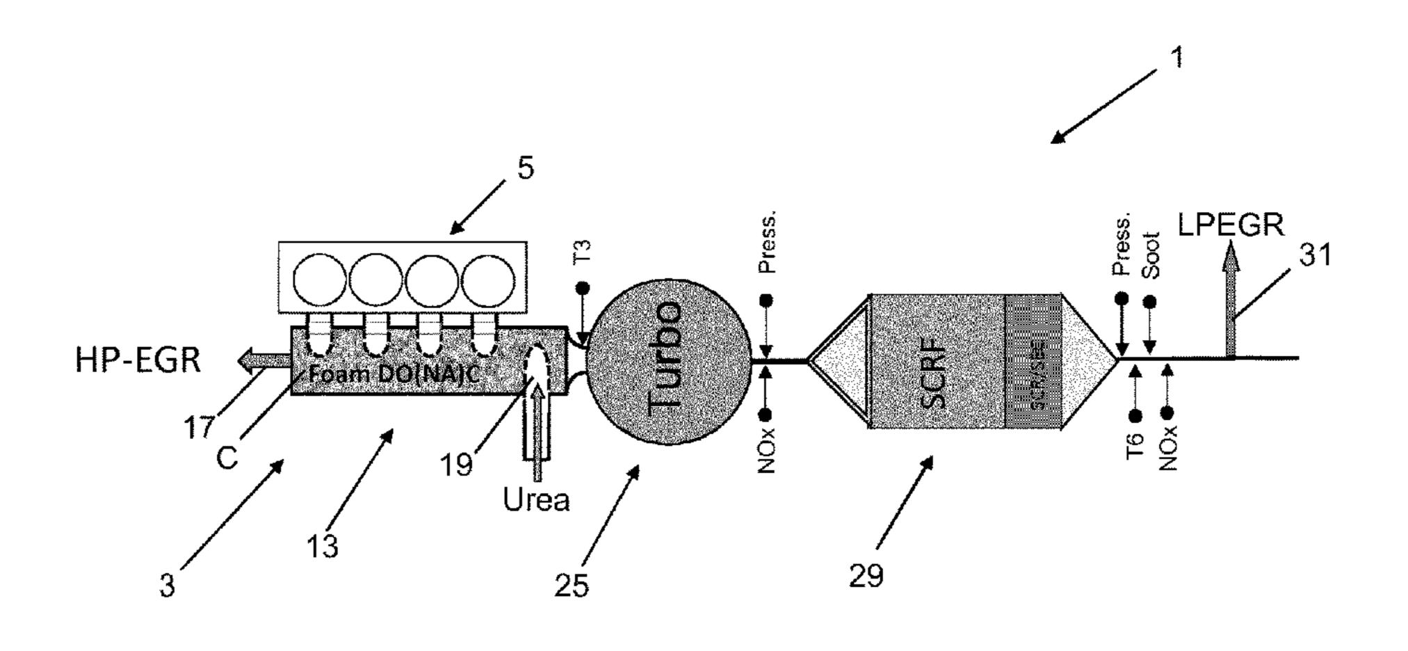
can have a three-dimensional open structure to facilitate the flow of exhaust gases. The invention also relates to a method of treating exhaust gases from an internal combustion engine (5).
