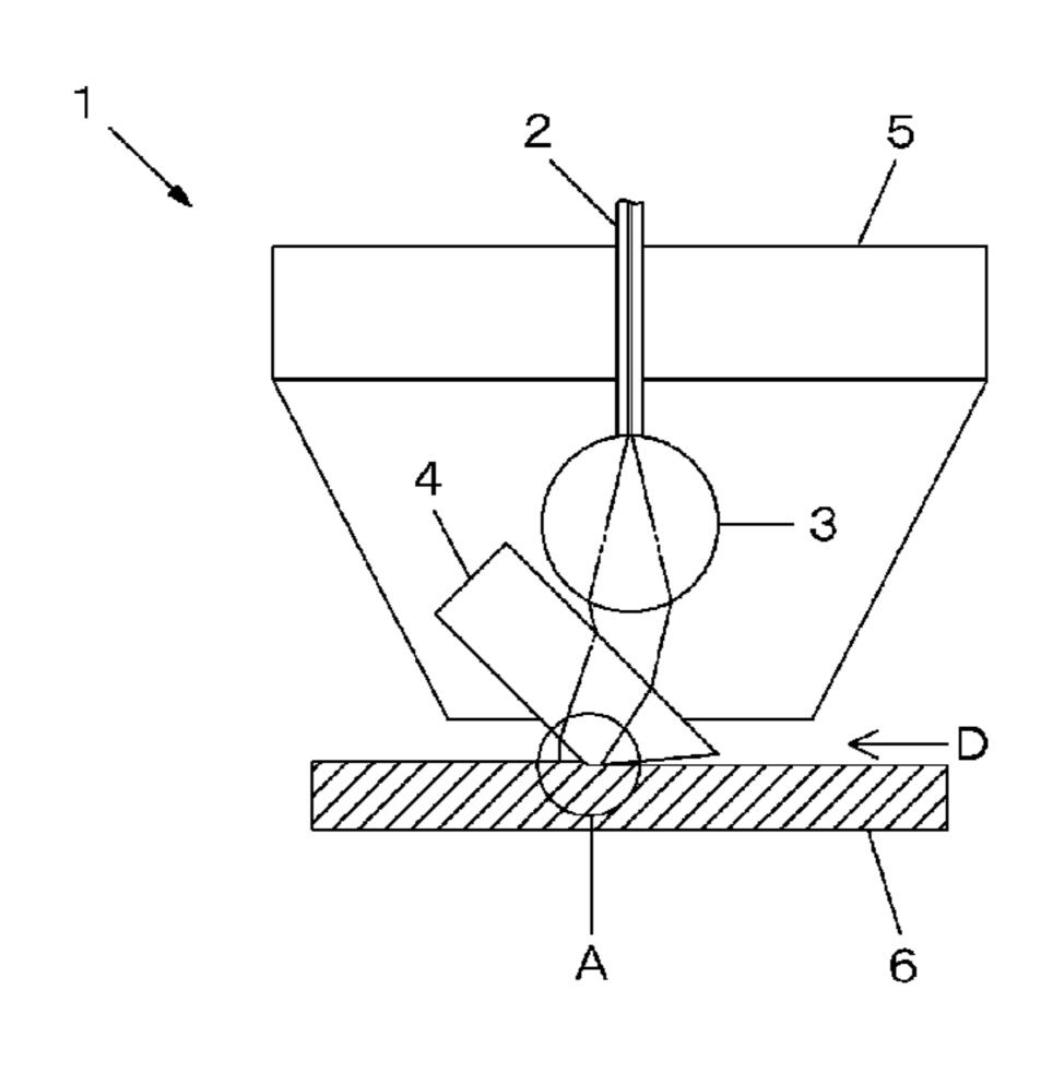
contact part and the rake angle part to soften the hard brittle material, and the softened hard brittle material is cut.
