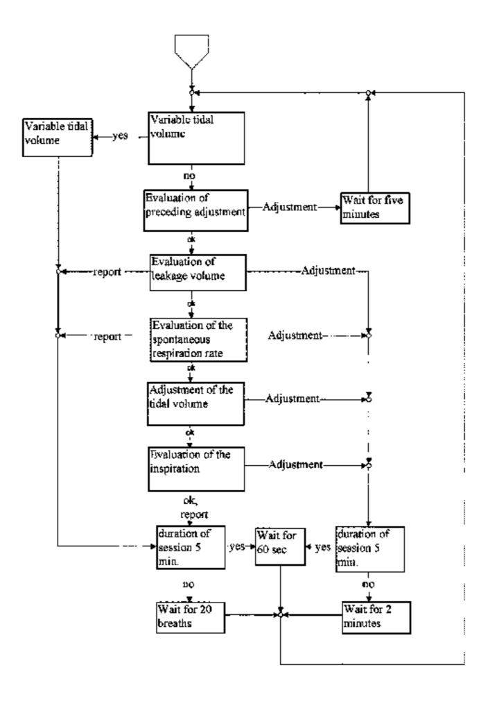
increases the inspiratory pressure and returns to I) or proceeds to step iii), iii) checks the volume and reduces or increases the inspiratory pressure and returns to I) or leaves the pressure assistance unchanged proceeding to step iv), iv) adjusts the time period of the pressure assistance, depending on the inspiration time, the time period being left unchanged if the inspiration time lies in the predefined inspiration time interval, and returns to I).
