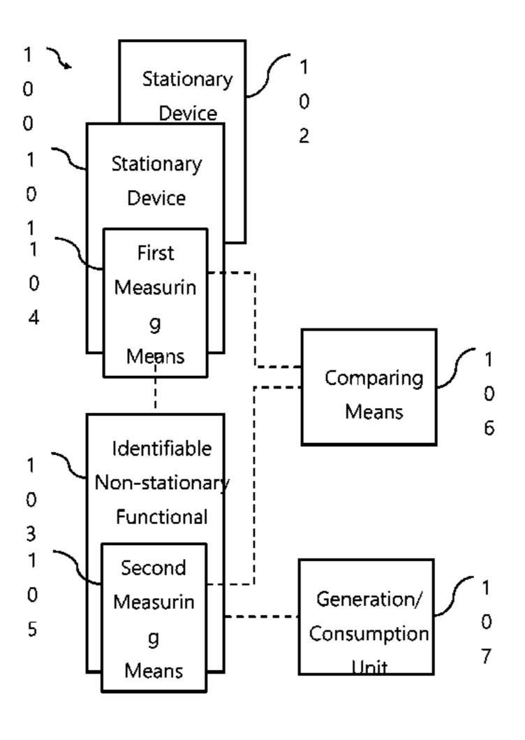
of feeding device further includes a comparing device configured to compare the at least one physical parameter measured at a connecting side with at least one physical parameter measured at a drawing off or feeding side.
