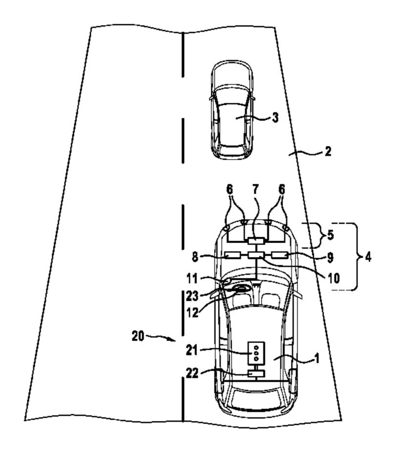
overtaking process has been detected, c) Actuating the drive device (20) to prepare the overtaking process in such a way that before the overtaking process is carried out a torque reserve of the internal combustion engine (21) is built up.
