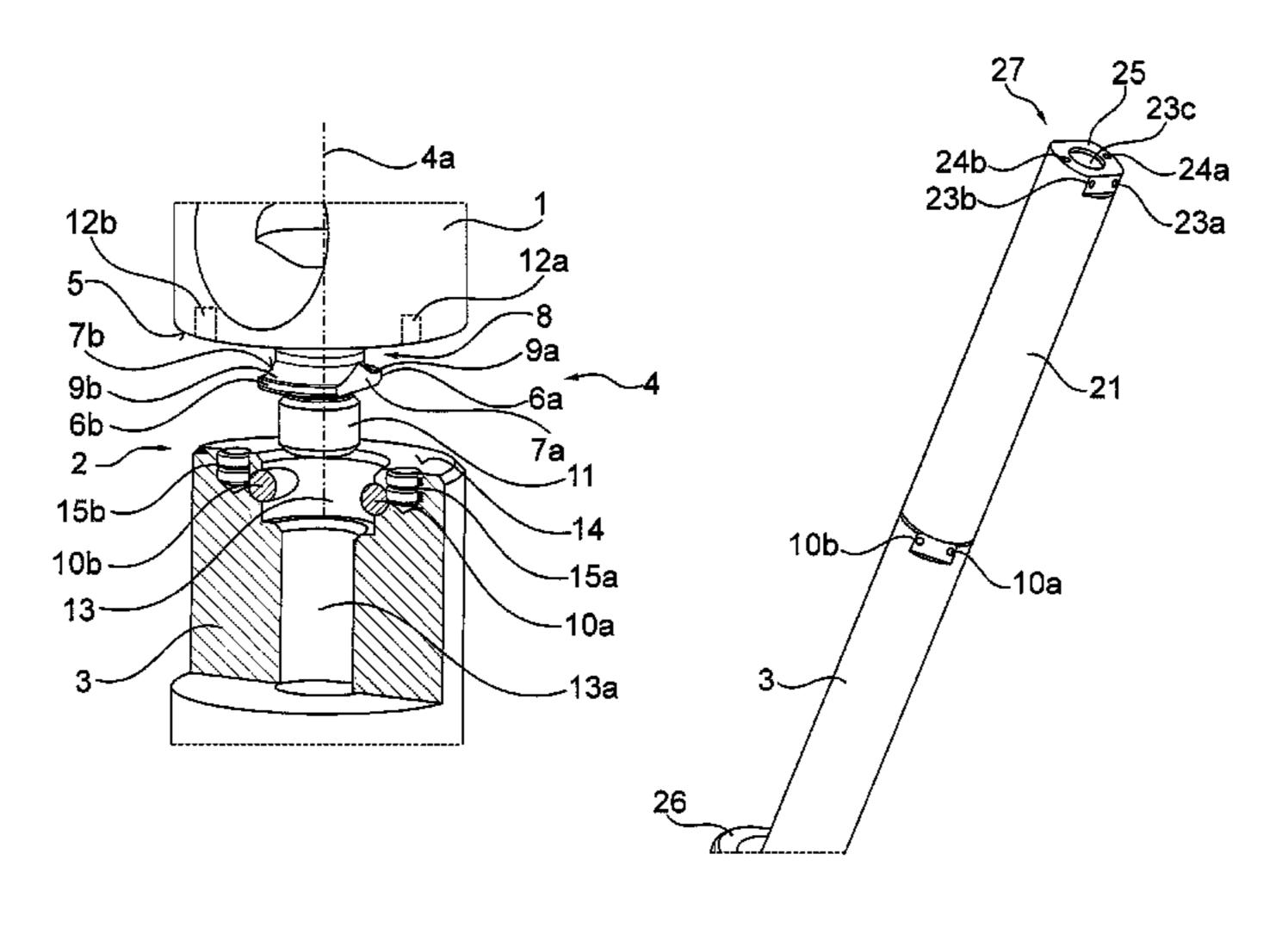
riveting tool can be releasably locked to the riveting tool receptacle by a magnetic force.
