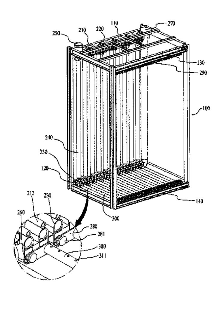
first lateral side; a first coupling unit provided at the first lateral side; and a second coupling unit provided at the second lateral side.
