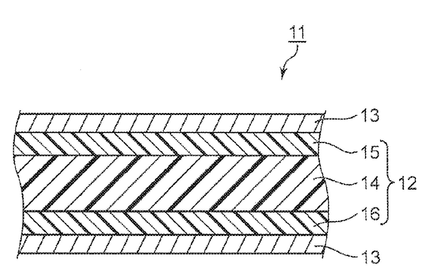
first resin layer and the second resin layer are smaller than a coefficient of thermal expansion of the cured product of the resin composition contained in the center layer.
