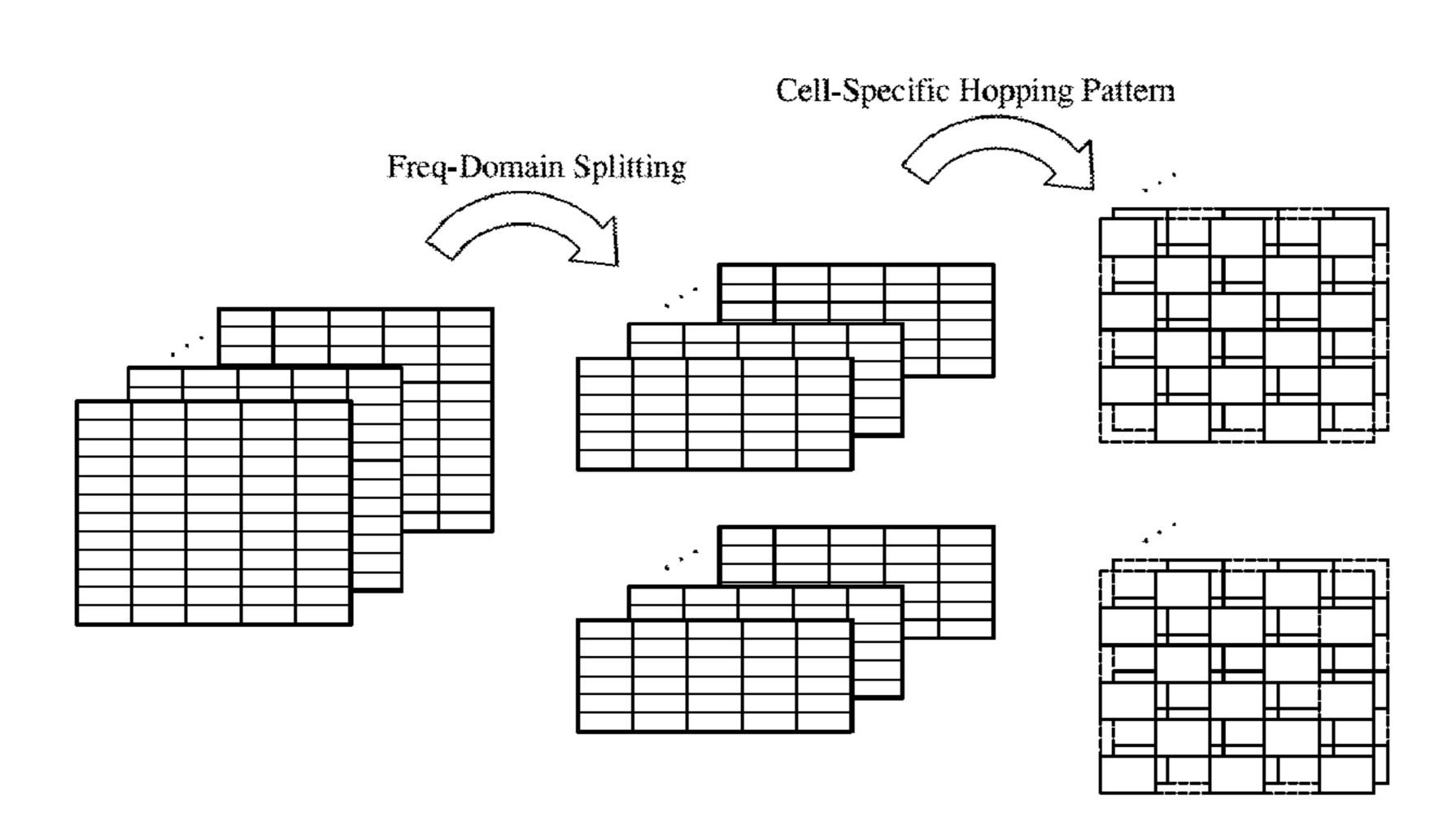
symbols. The transmitted uplink reference signal is hopped in the frequency domain, based on a cell specific hopping parameter.
