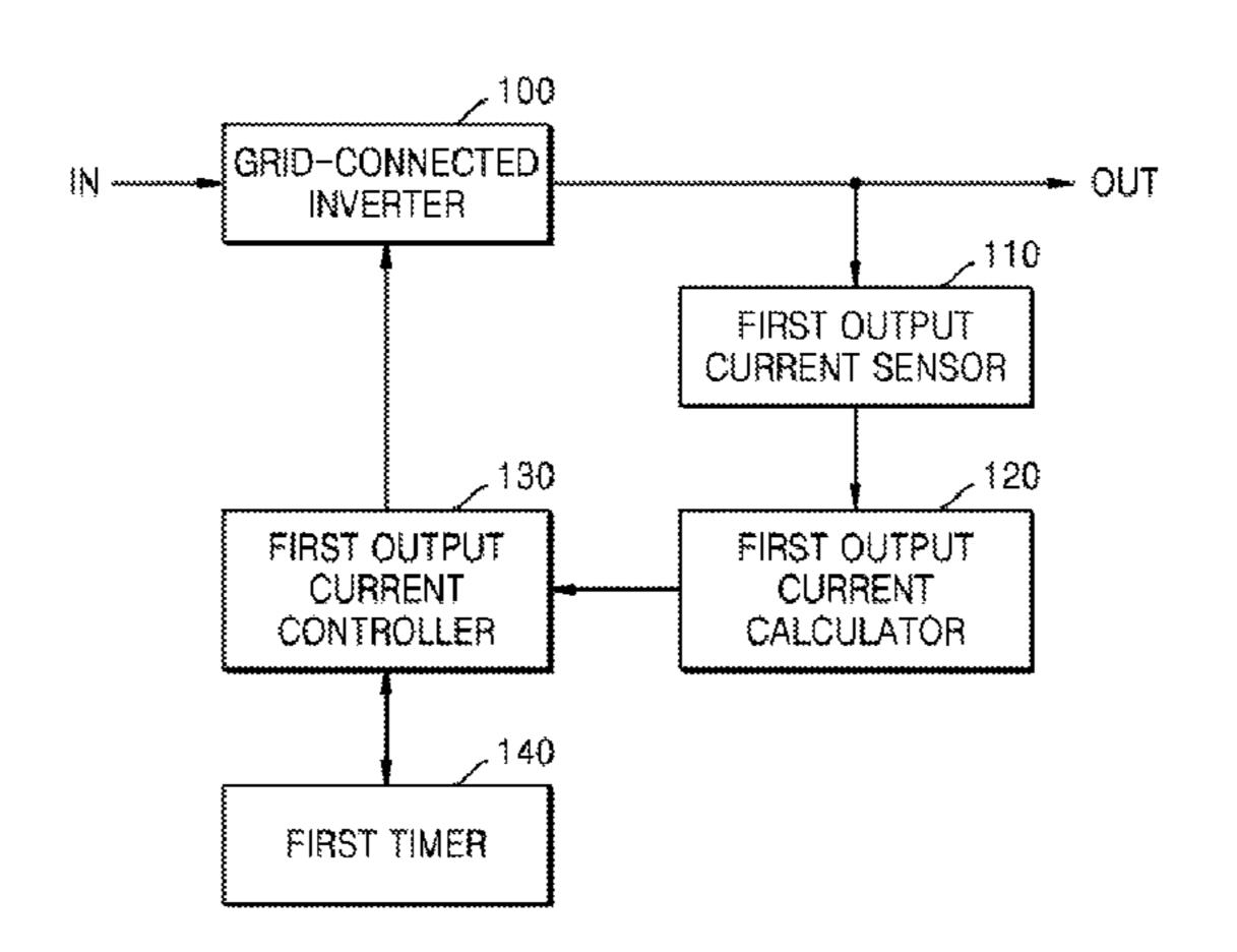
current by a predetermined value when the difference between the output current and the reference current exceeds the predetermined range.
