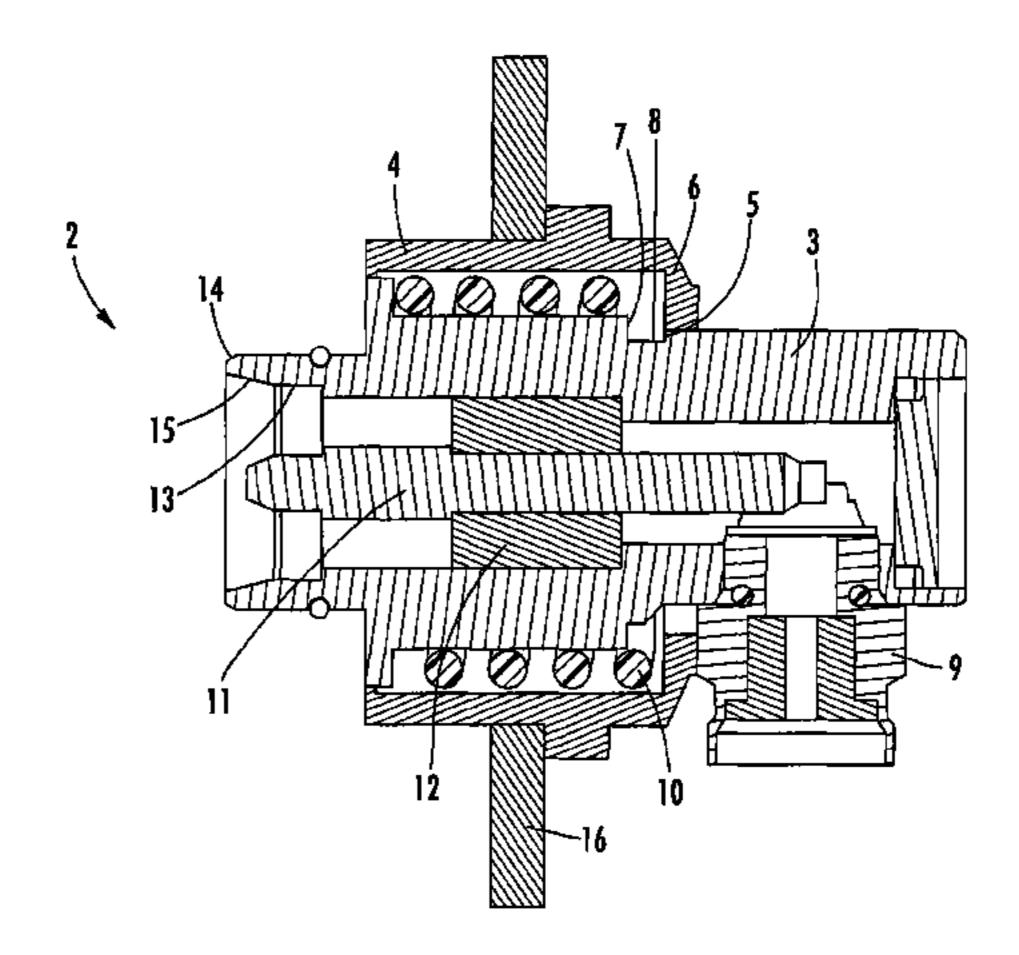
first connecting device and the second connecting device are brought together, without necessarily making the first connecting device and the second connecting device be axially aligned precisely with each other. The present invention allows relative floating of connecting devices of a plurality of pairs of low-intermodulation RF connectors, allows simultaneous quick blind mating connection, and improves connecting efficiency and installation reliability.
