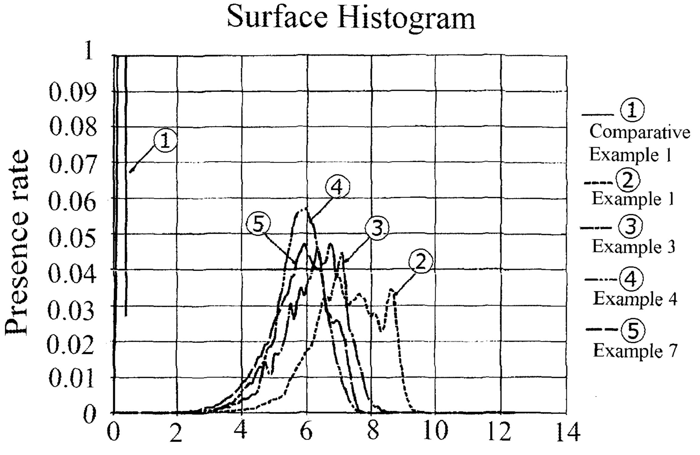
Heights of indentations and protrusions in the surface  $(\mu m)$
