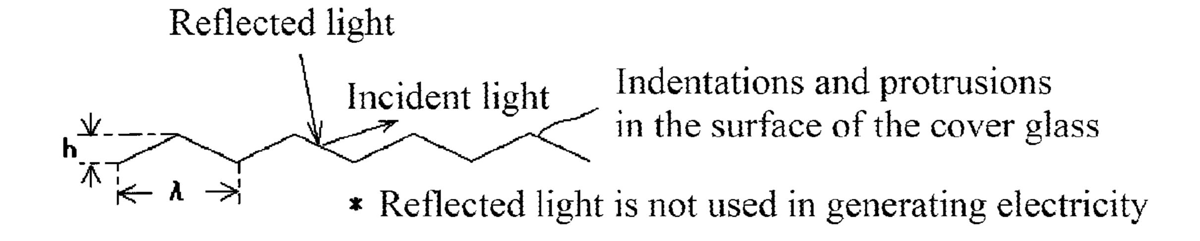
Indentations and protrusions in the surface  $\theta$  \*When an angle  $\theta$  is  $\theta$  < critical angle (41.47°), reflected light is totally reflected.
