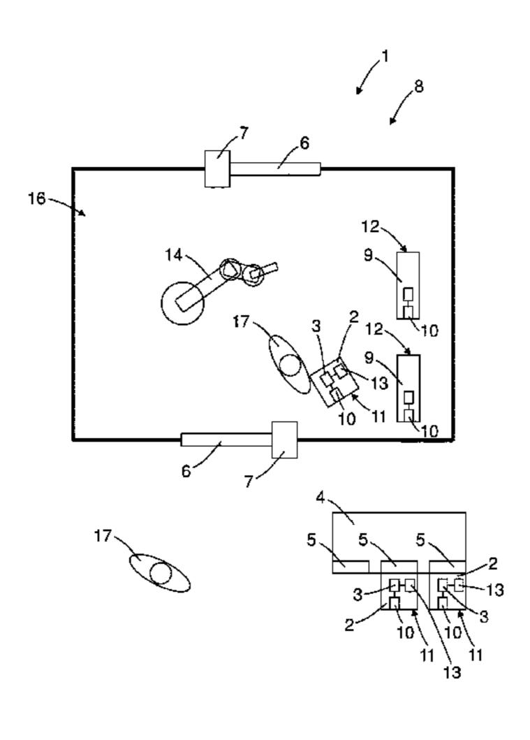
the facility (8) being deactivated or blocked when at least one key unit (2) has been removed from the key station (4).
