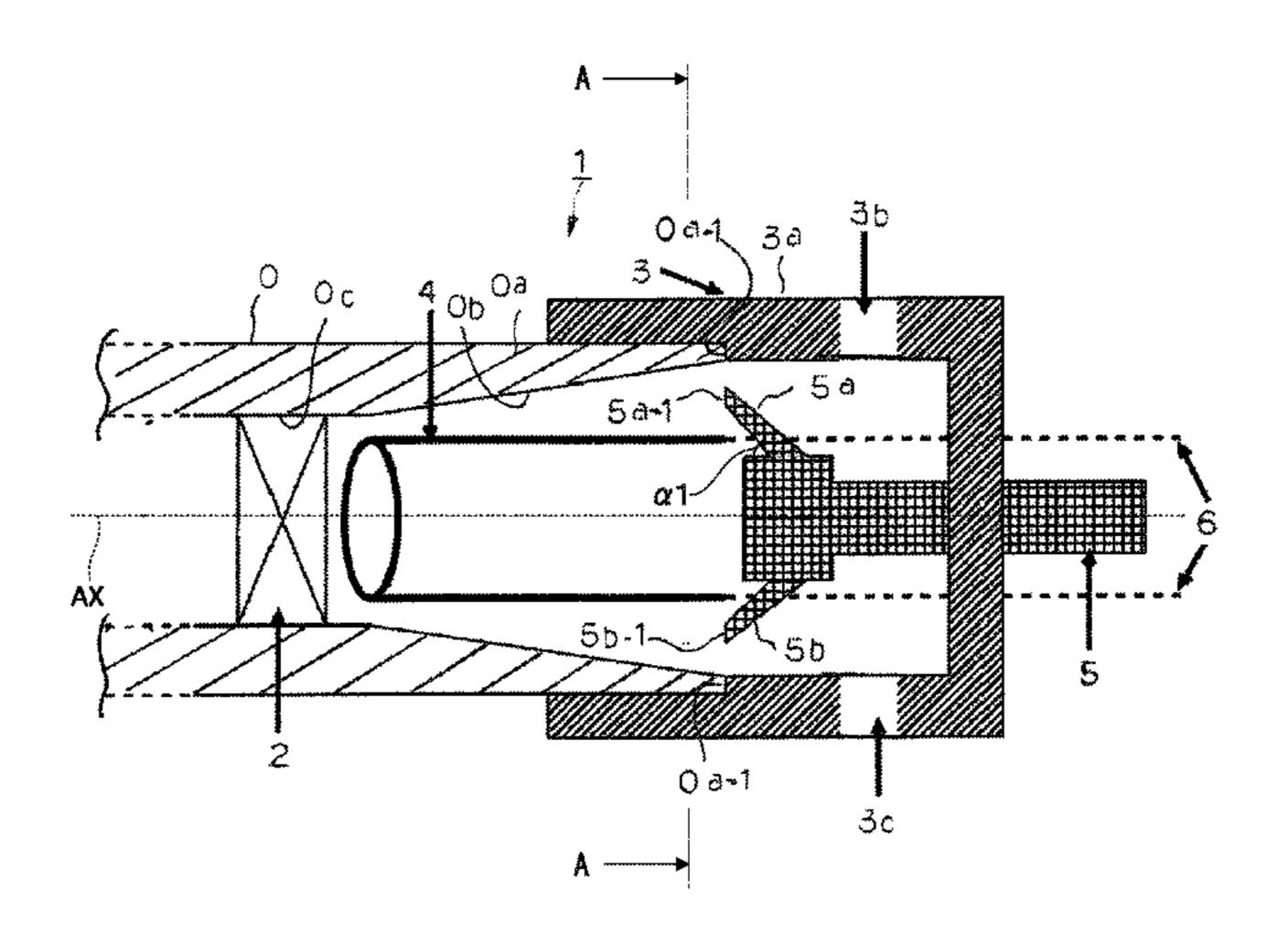
nozzles thereinside and is mounted to the pipe end, when viewed in the pipe axial direction, a tip of each of the nozzles is positioned between the female screw and the insoluble electrode, and each of the nozzles injects the plating solution toward a direction which intersects an extension direction of the nozzle, the direction being a rotational direction of a clockwise direction or a counterclockwise direction in which the pipe axis is the center.
