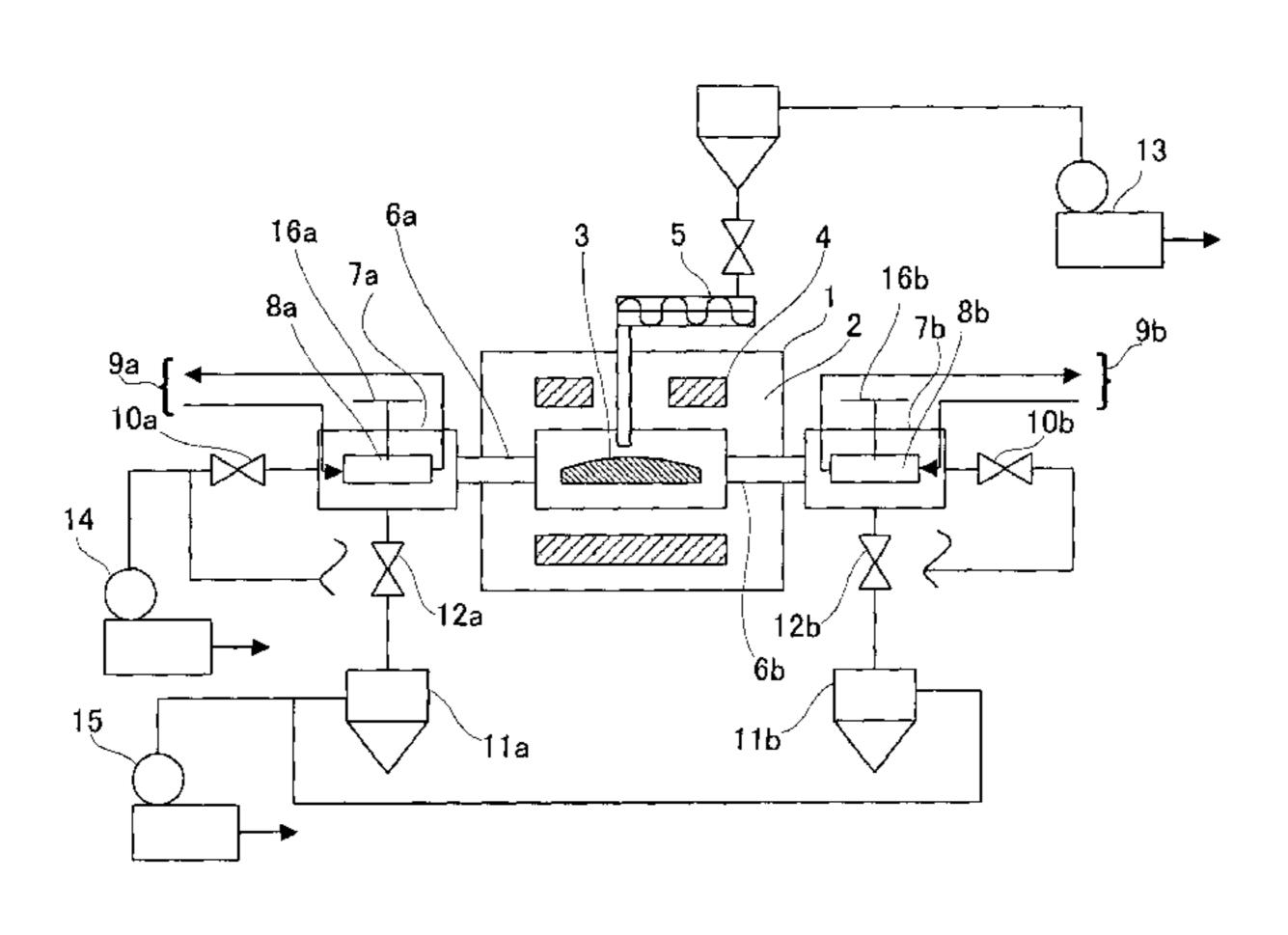
and the step of delivering the vapor is alternately switched from one to another deposition chamber.
