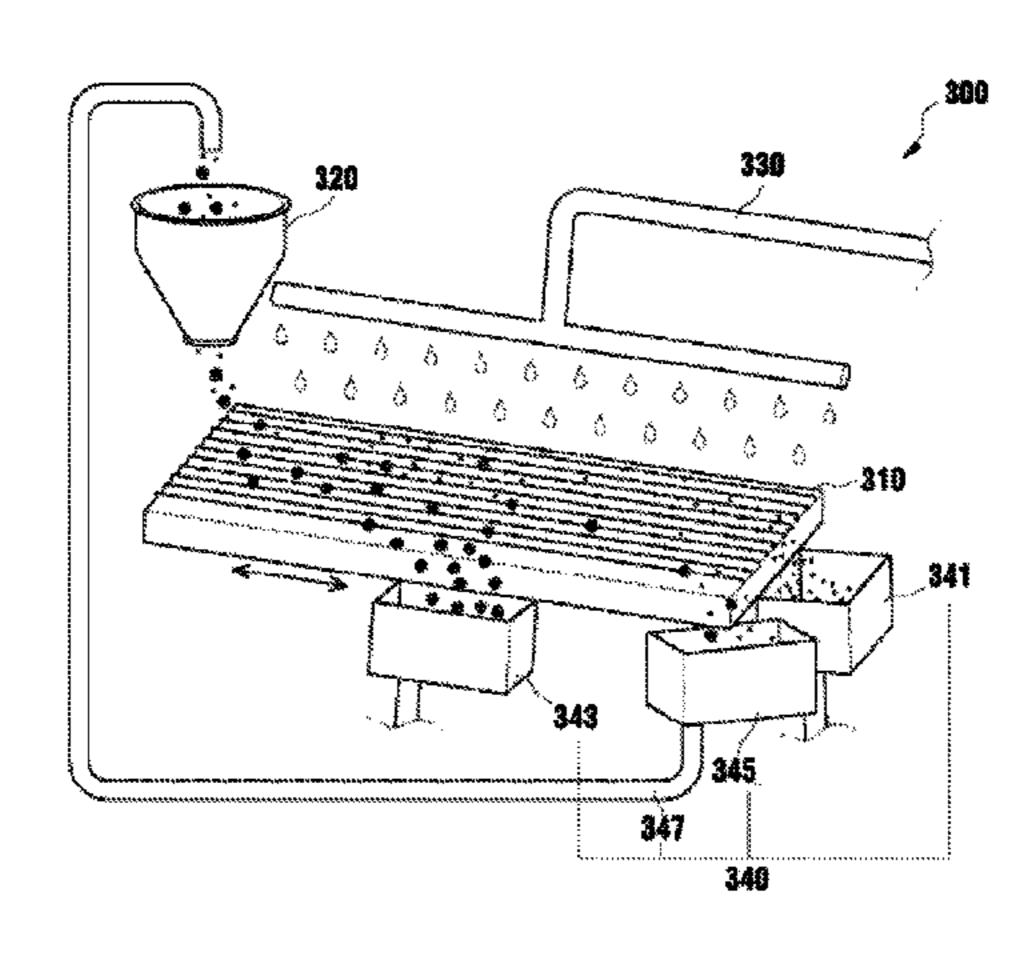
on a grain size; and a second sorting operation of sorting the materials, which are sorted by the first sorting operation and have grain sizes belonging to a predetermined range, based on specific gravity.
