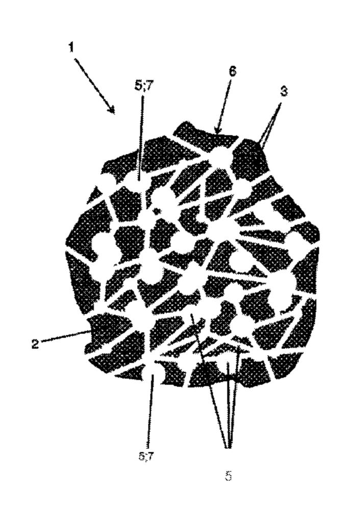
sorption material, in which pores are introduced into the granules by means of a porosity agent during the production.
