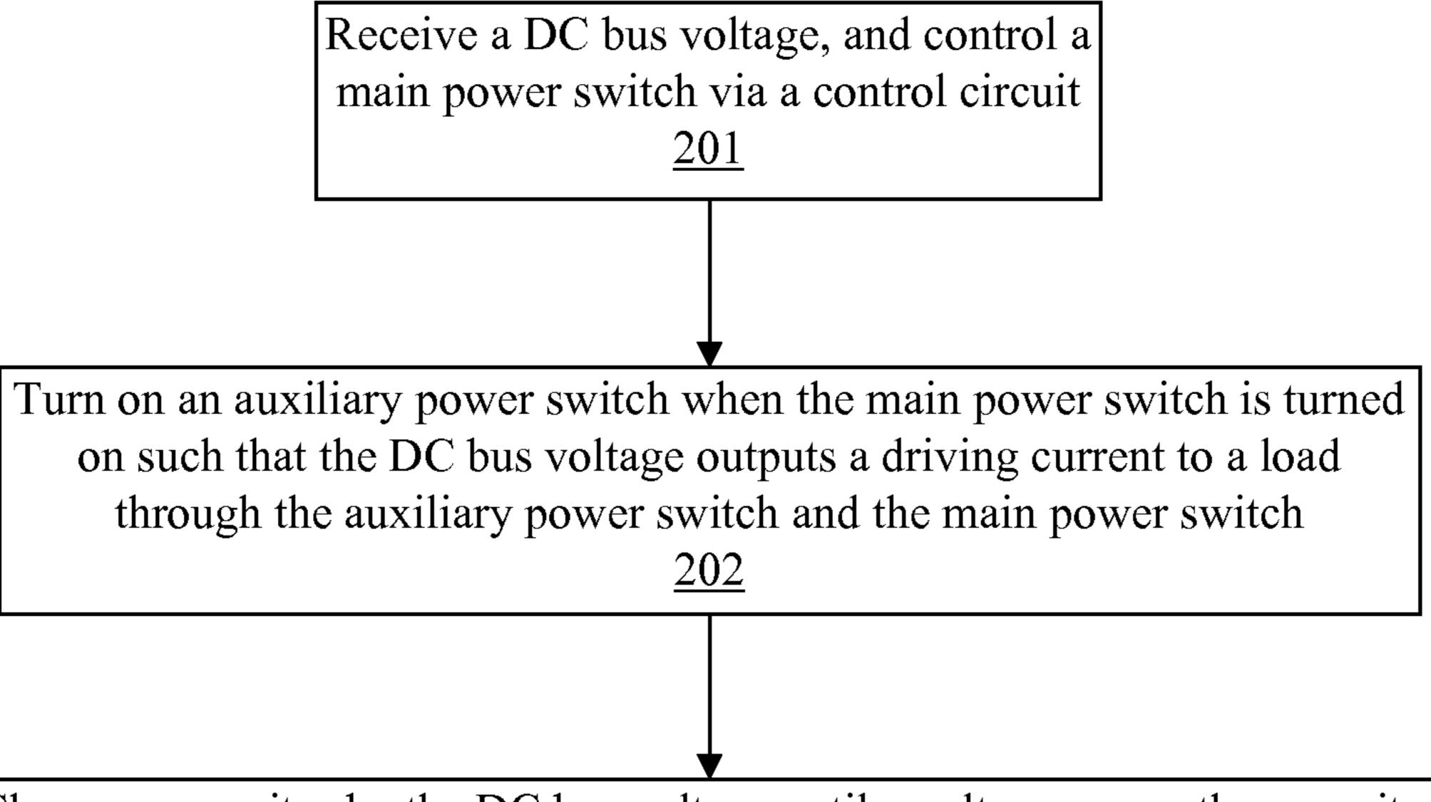
Charge a capacitor by the DC bus voltage until a voltage across the capacitor reaches a predetermined stable voltage when the main power switch is turned off, and clamp the voltage across the capacitor to a stable voltage  $\frac{203}{}$
