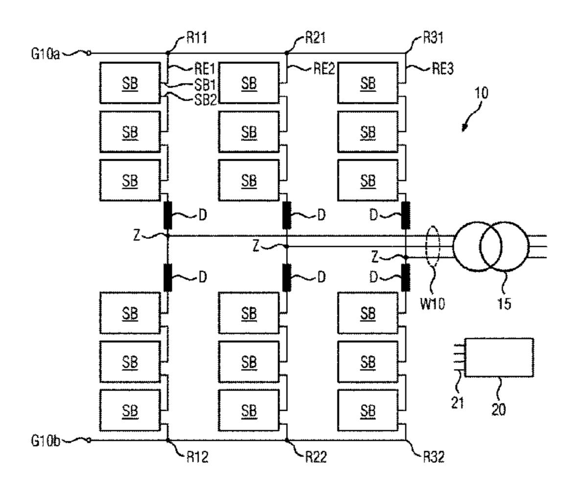
capacitor, and a first and a second part-module terminal. The galvanic connection between the two part-modules includes at least one inductive element.
