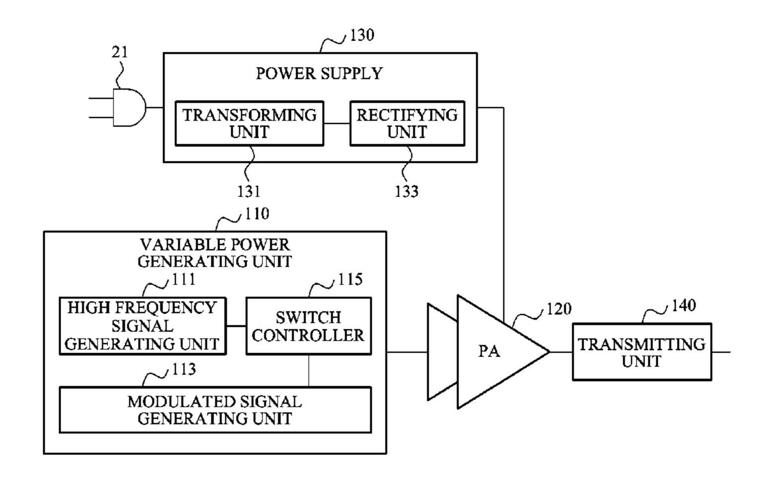
(DC) voltage, generating the supply voltage having the predetermined level based on the DC voltage, and providing the supply voltage having the predetermined level to the PA.
