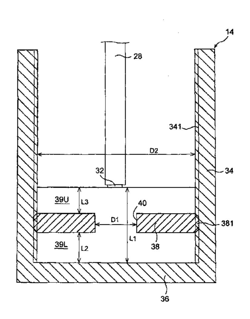
through hole and is positioned below a liquid surface of the SiC solution when the SiC solution is contained in the crucible.
