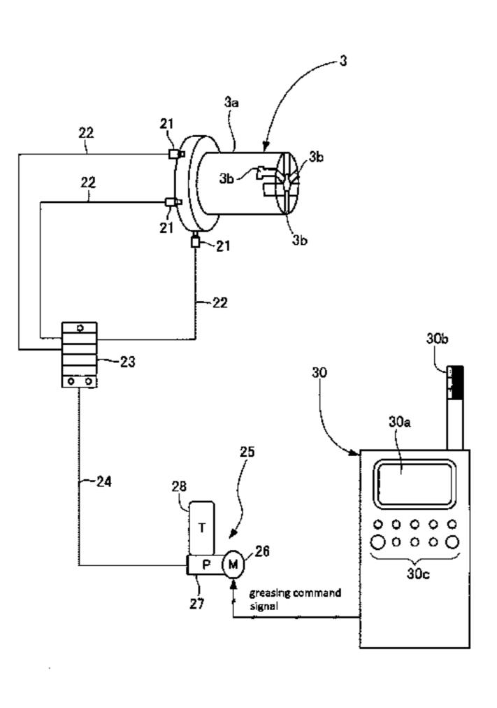
command signal output unit (33); and a notification means (30a, 30b) for notifying that a cutter (7) needs replacement in response to a notification command signal output unit (36) which has received the rotary cutter replacement command signal as the trigger signal from a rotary cutter replacement command signal output unit (33).
