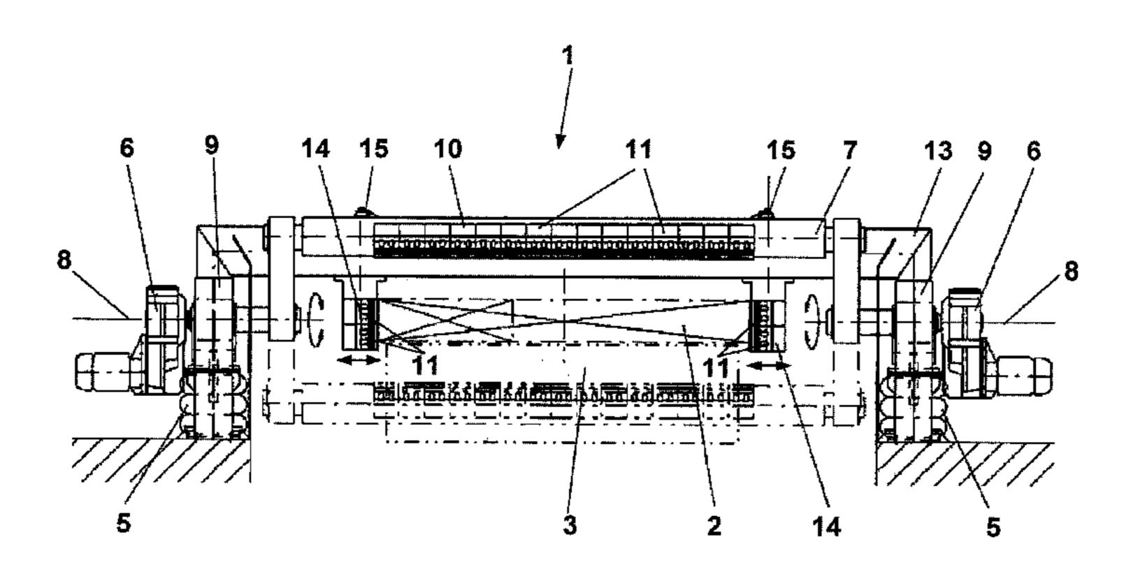
approximately 180° on a horizontal axis (8) around the top, bottom and cut sides of the work piece (2) by means of a swivelling drive (6) while the work piece is moved back and forth.
