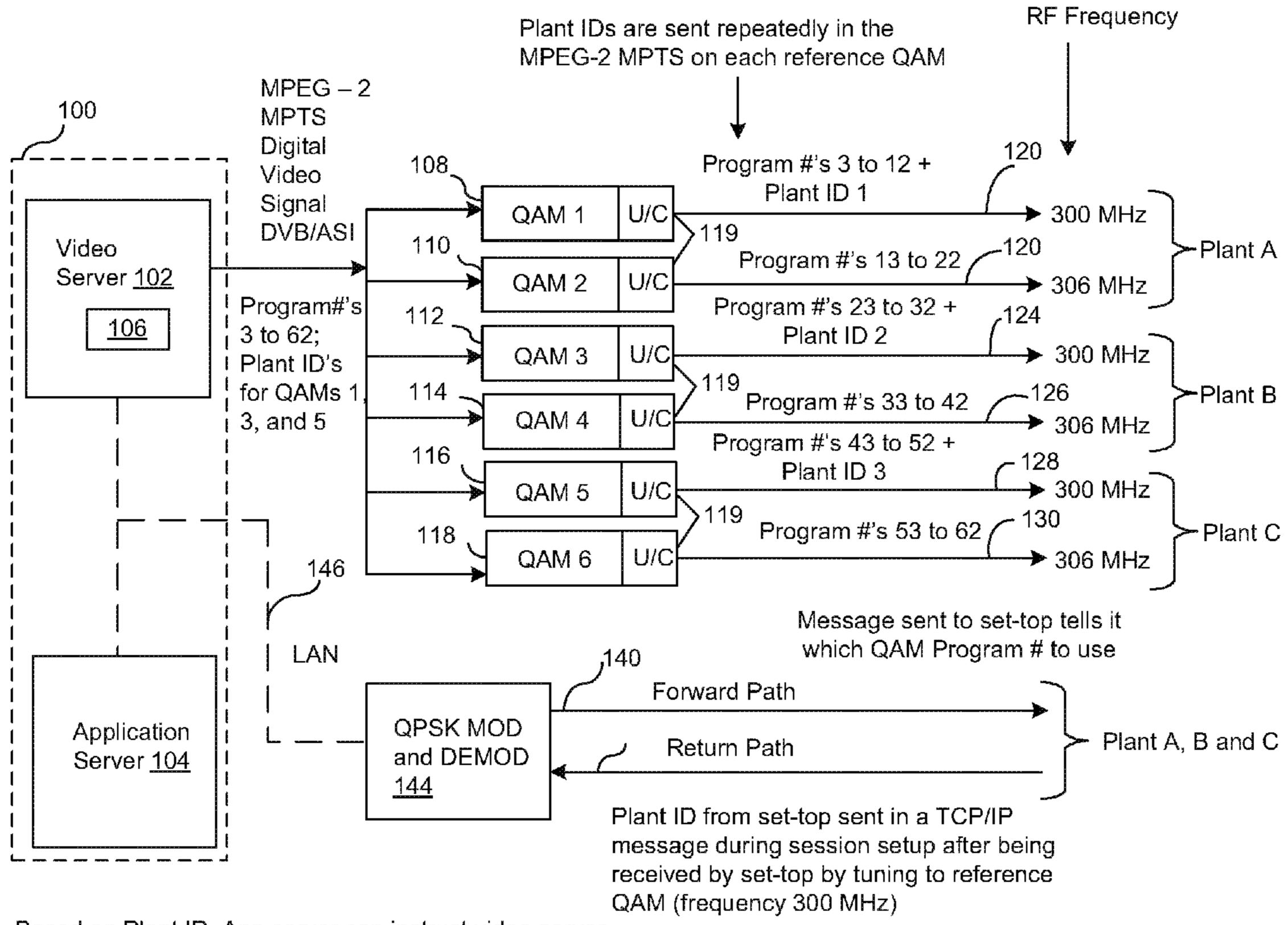
Based on Plant ID, App server can instruct video server which QAMs and Program #s cab be used to send the video program to the set-top. It can tell the set-top as well.
