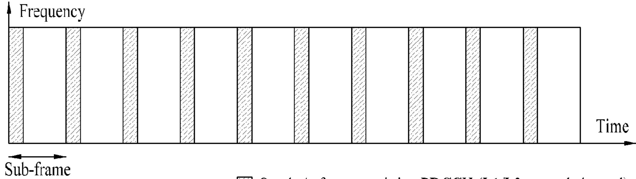
Symbols for transmitting PDCCH (L1/L2 control channel)
