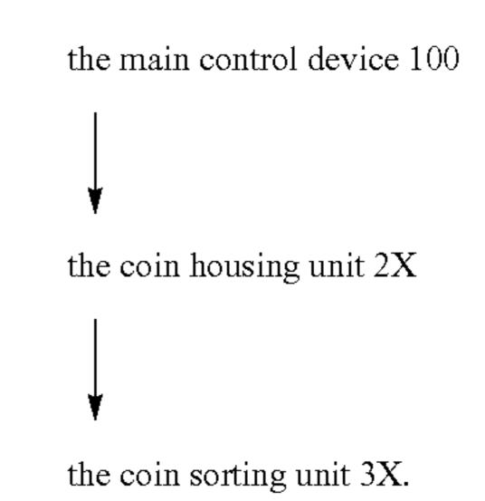
In contrast, a flow of power source supply of the low-voltage power source is as follows:
