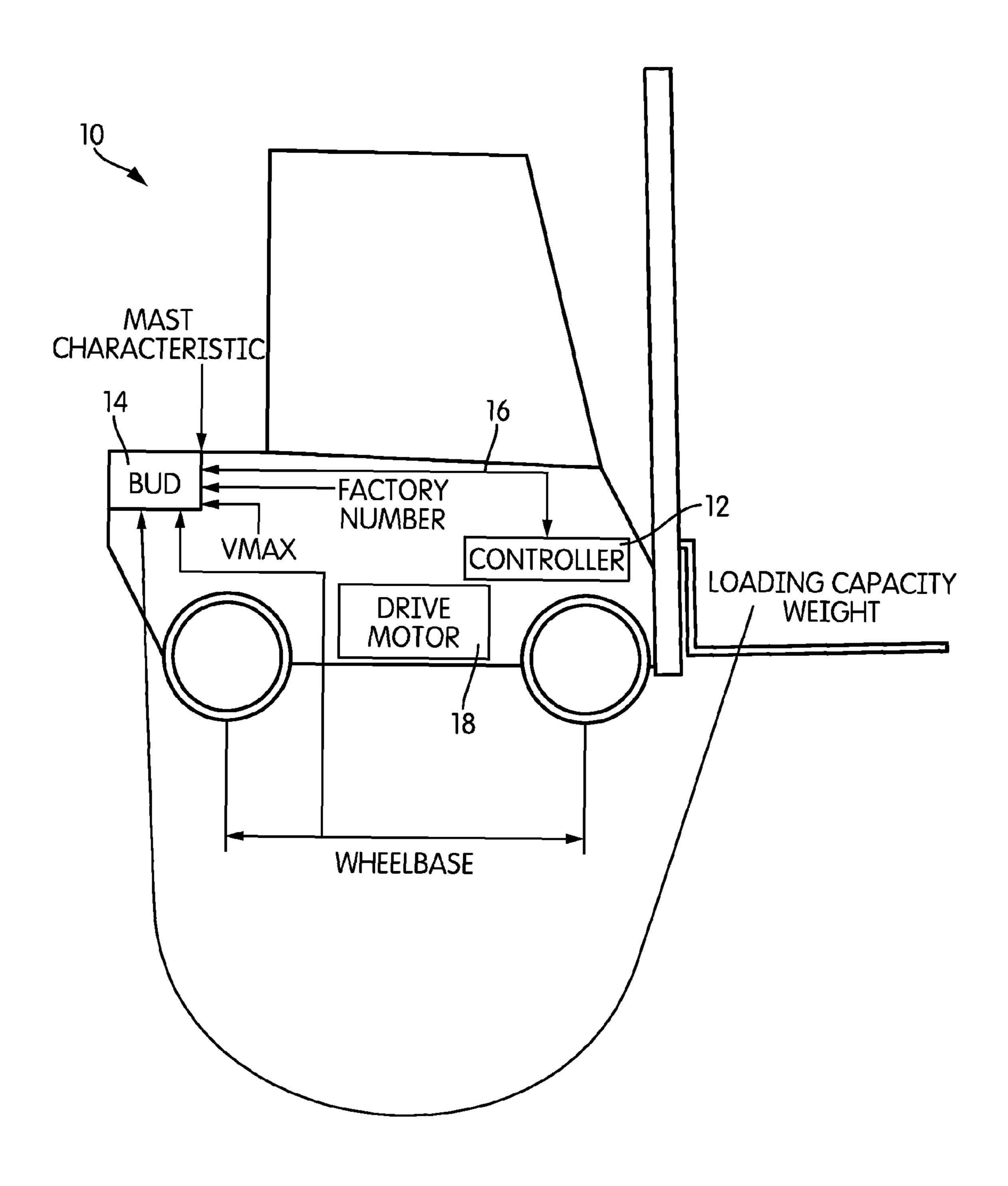
COMMERCIAL VEHICLE, IN PARTICULAR FORK-LIFT TRUCK OR INDUSTRIAL TRUCK, WITH A DATA MEMORY THAT IS RIGIDLY ATTACHED ON THE VEHICLE SIDE AND ASSIGNED TO A PARAMETERISABLE ELECTRONIC CONTROL ARRANGEMENT
