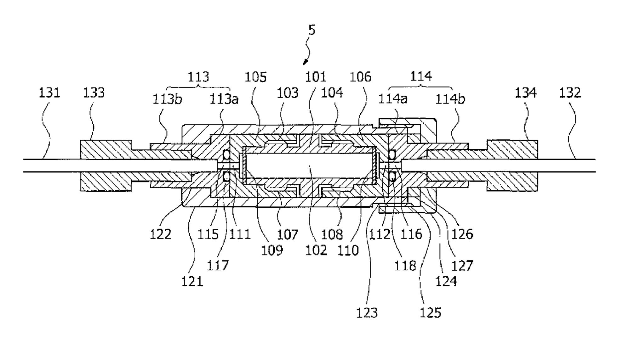
members (113, 114) in an engaged state. A cover member (124) is detachably installed on a side of an opening of the case (121).
