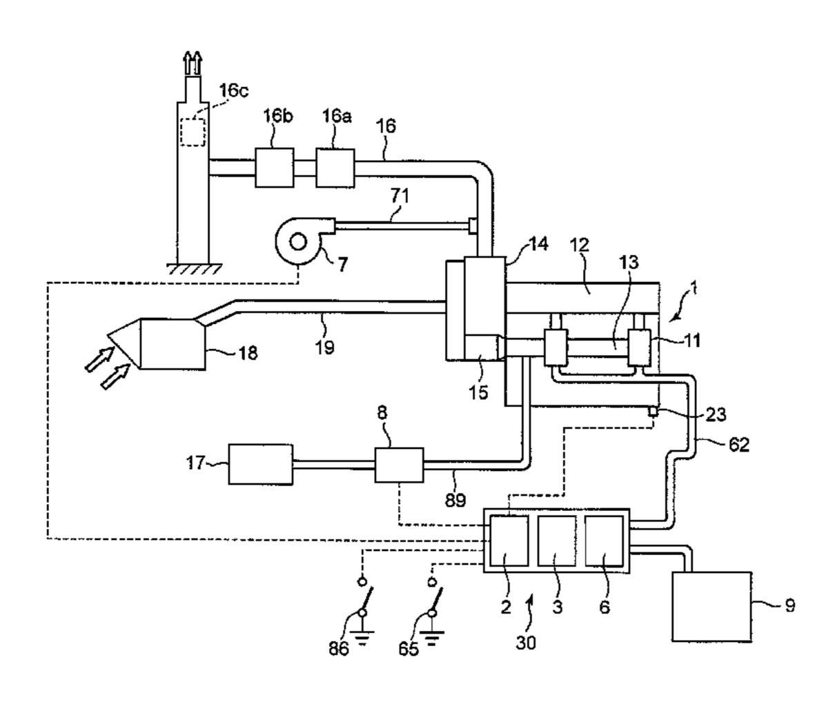
ambient air to the exhaust channel 16, and a control device 2 for performing a control to drive the exhaust purge fan 7.
