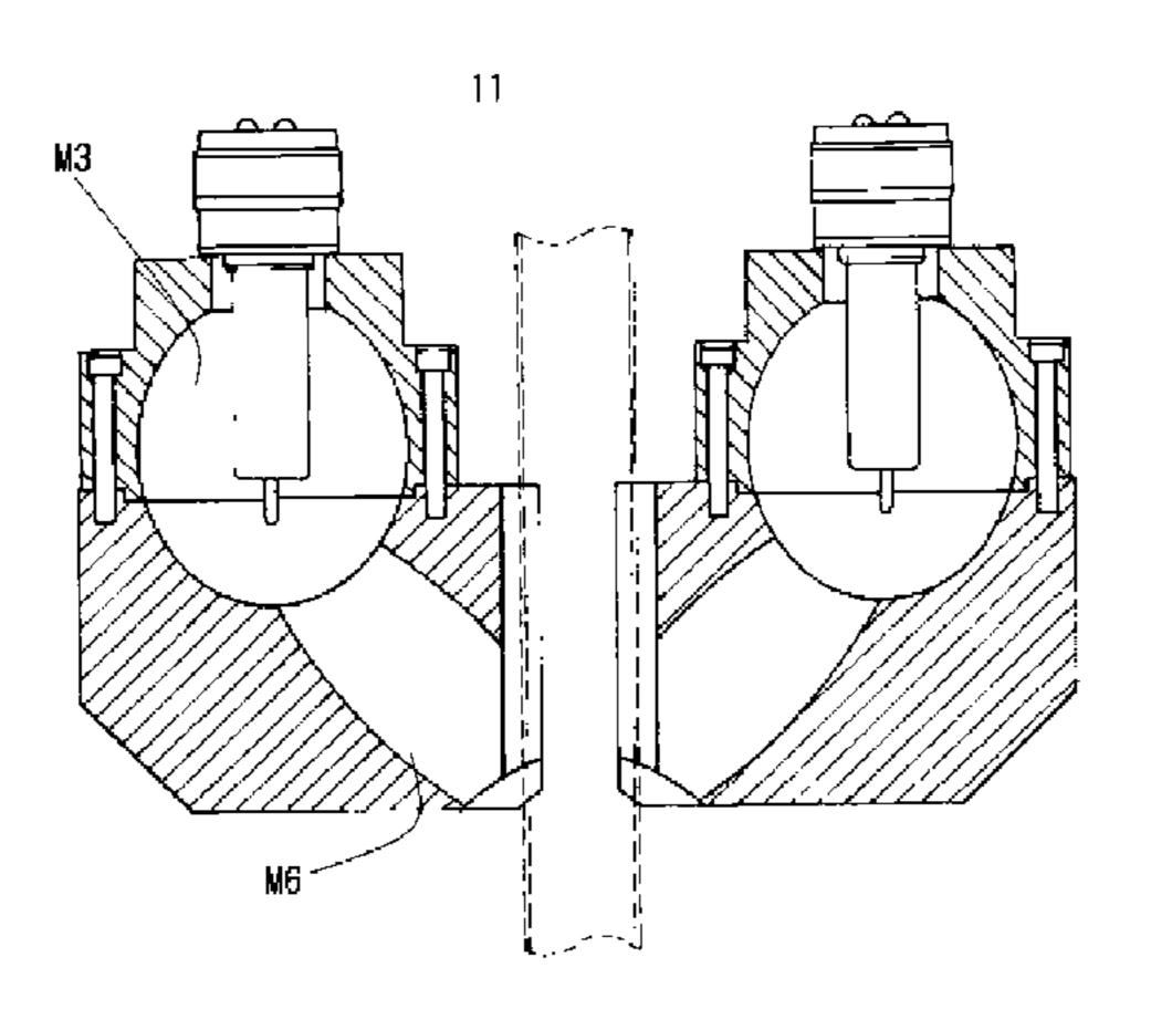
sequentially by the primary reflecting mirror and secondary reflecting mirror and then irradiated onto the target; and the light reflected by the secondary reflecting mirror and irradiated onto the target surface is not perpendicular to the target surface. Based on the above, a system that uses converged infrared light to provide heating can be made smaller while keeping its heating performance intact, even when the system uses a revolving ellipsoid.
