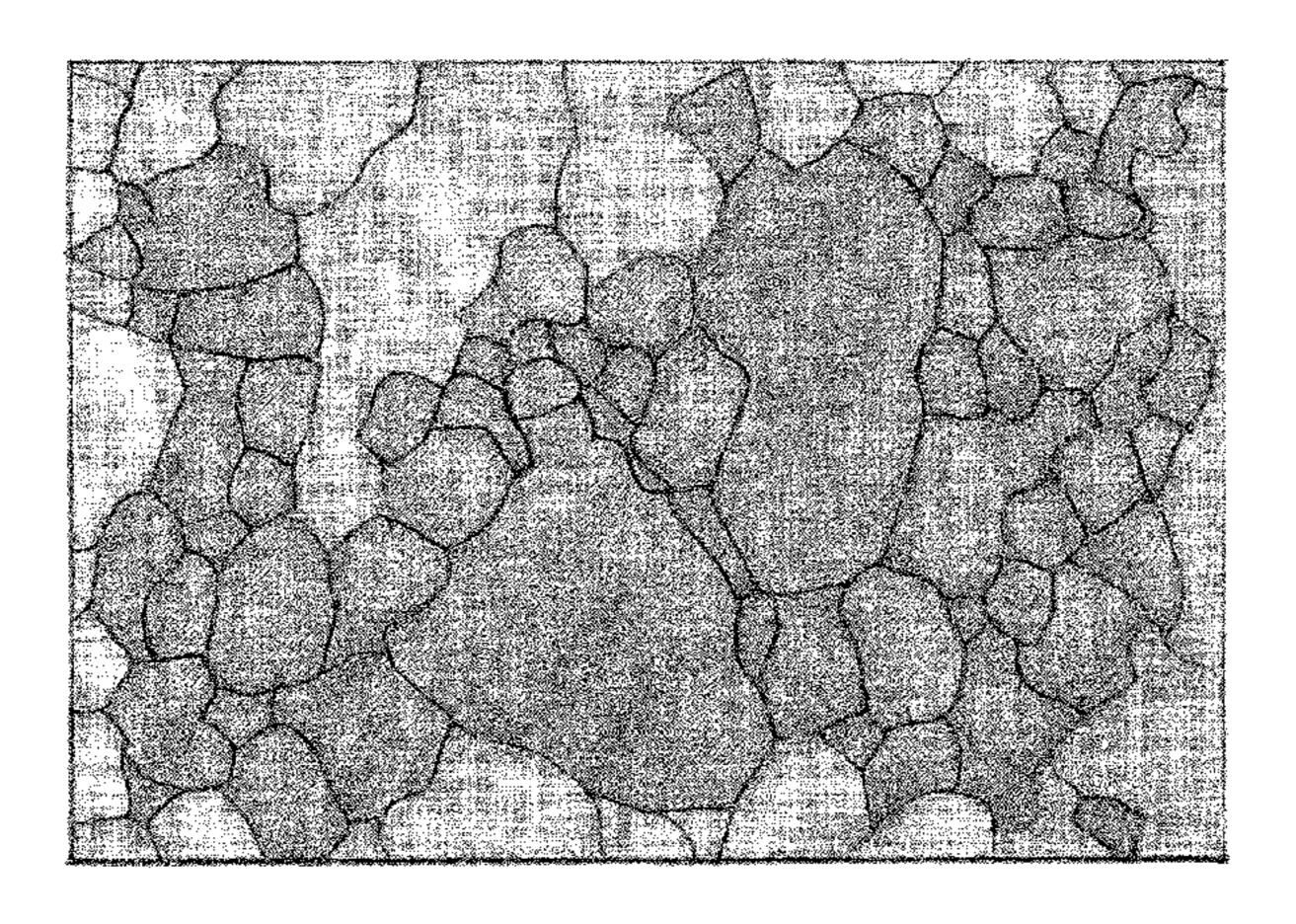
class, rate of cross-sectional area of zirconia crystal-grains in class of <0.4  $\mu$ m is 4% to 35%, rate of cross-sectional area of zirconia crystal-grains in class of  $\geq$ 0.4 and <0.76  $\mu$ m is 24% to 57%, and rate of cross-sectional area of zirconia crystal-grains in class of  $\geq$ 0.76  $\mu$ m-is 16% to 62%.
