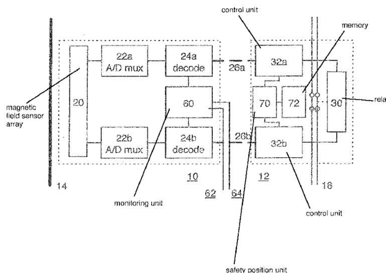
the emergency function can be activated as a response to the position or speed signal and to the elevator car status signal if a car movement with the elevator car door open exceeds a predetermined speed threshold value and/or acceleration threshold value and/or displacement threshold value.
